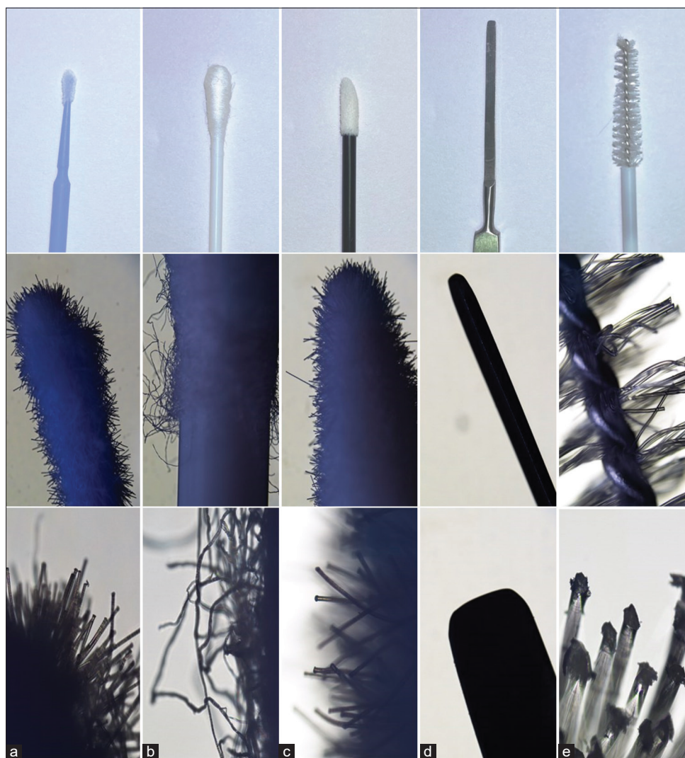
Figure-1: Cytological sampling instruments in native size. Line 1 (a) mini brush, (b) cotton swab, (c) soft brush, (d) spatula, (e) cytobrush. Line 2 (magnified 20×). Line 3 (magnified 100×).
